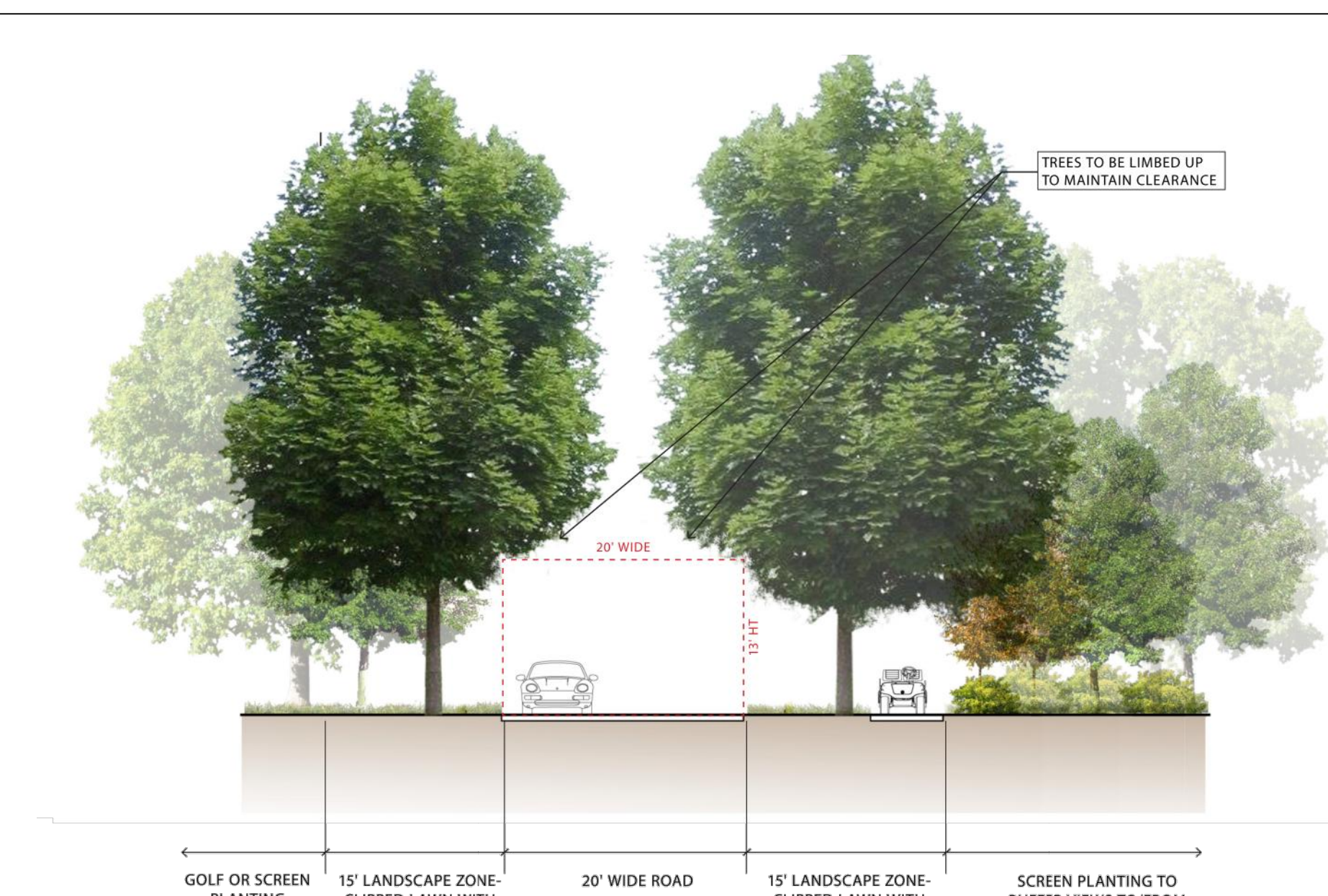
SECTION B TYPICAL STREET SECTION
